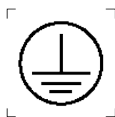
Figure 5 – Symbol IEC 60417-5019: Protective earth
