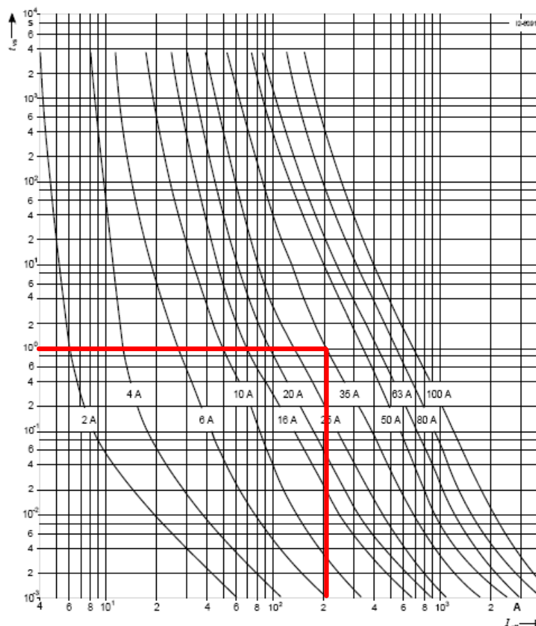
Zeit-Strom-Kennlinien-Diagramm/Time-current characteristic chart Diagramma della curva caratteristica tempo-corrente/Tid-ström-diagram
